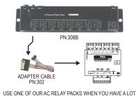
OF 110 VOLT DEVICES TO CONTROL. THE OUTPUTS ON THE RELAY PACK WILL MIRROR THE OUTPUTS ON THE FLEX.
