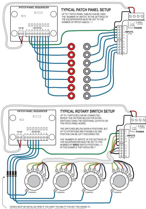
DIODES MUST BE INSTALLED HERE IF YOU WANT THE ABILITY FOR ANY TWO KNOBS T BE IN THE SAME POSITION FOR THE SOLUTION. FOR EXAMPLE, IF YOU WANT THE SOLUTION TO BE 1,2,3,1, YOU WOULD NEED DIODES. IF YOU ARE OK WITH 1,4,3,2 OR 4,2,1,3, ETC. THEN YOU DON'T NEED THEM.
