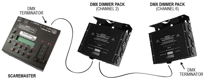
Typical DMX Master Mode Network
